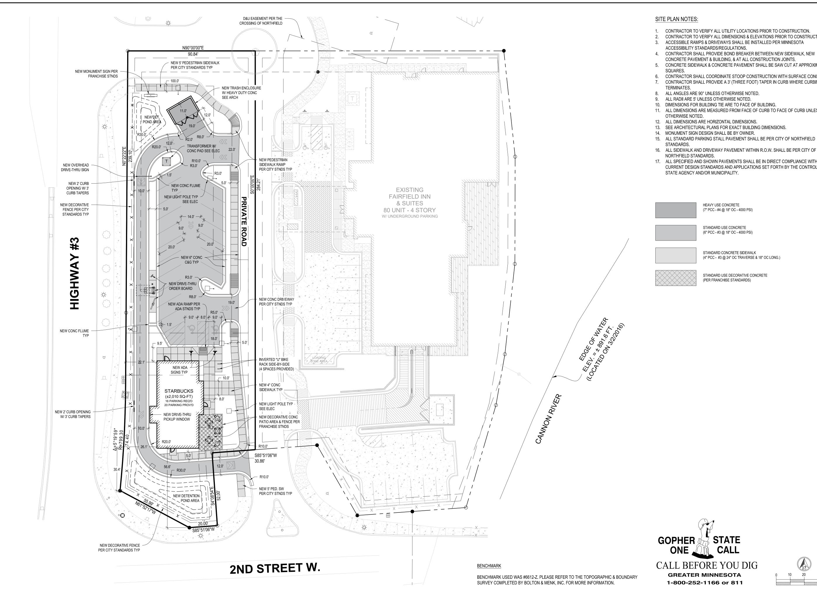
CONTRACTOR TO VERIFY ALL UTILITY LOCATIONS PRIOR TO CONSTRUCTION. CONTRACTOR TO VERIFY ALL DIMENSIONS & ELEVATIONS PRIOR TO CONSTRUCTION. ACCESSIBLE RAMPS & DRIVEWAYS SHALL BE INSTALLED PER MINNESOTA ACCESSIBILITY STANDARDS/REGULATIONS.
